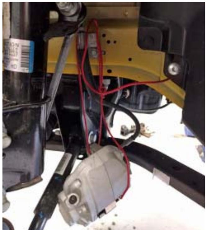
6. Remove the brake rotor and set aside.
