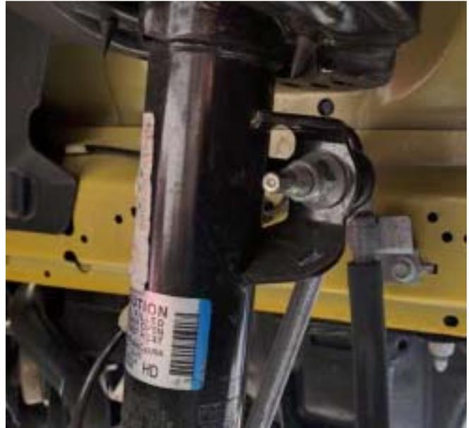
5. Using a 15mm socket remove the two caliper to spindle bolts holding on the caliper. Do not let the caliper drop or hang from the brake hose. We recommend securing it the brake hose to chassis bracket like shown in the photo.
