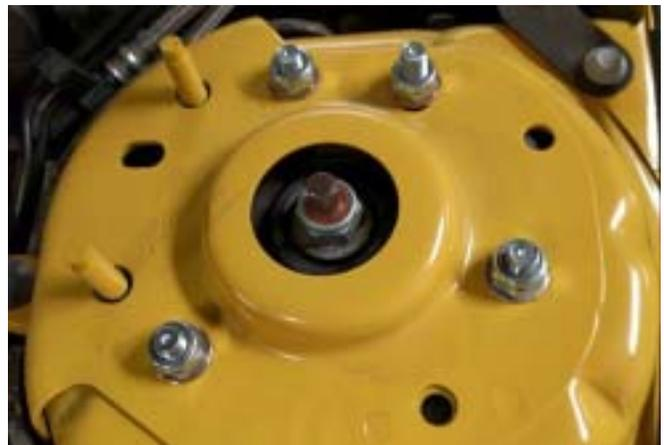
18. Attach the strut to the spindle. Make sure to install the strut to spindle bolts from the front side of the spindle.
