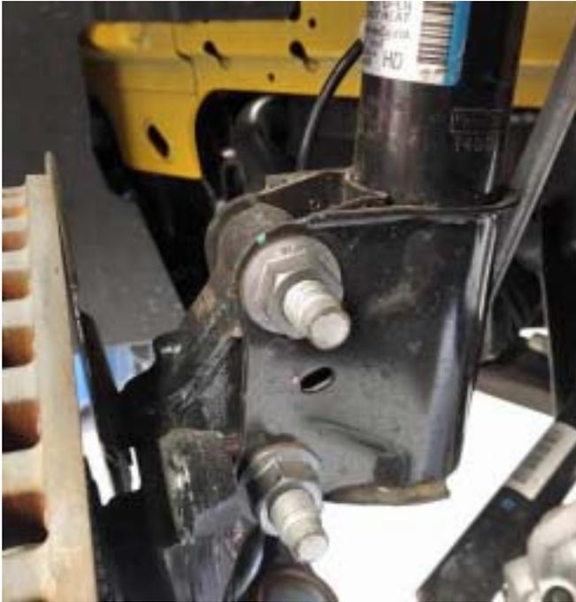
8. Carefully using a hammer hit the end of the strut to spindle mounting bolts to drive them out. These bolts are splined so it will take some force to get them out.
