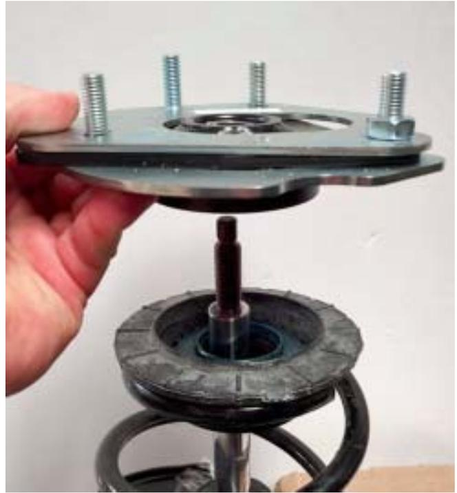
15. If using the OEM strut re-install the nut and torque to 76 lb/ft. Do not use an impact gun. If you are using an aftermarket strut, torque to the manufacturer's recommended torque specifications.
