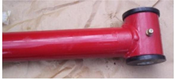
Step 6. Install the grease fittings into the arms by tapping on them. Be sure to tap straight down so the fitting gets installed properly. They are press fit, so once they are tapped into place you are finished.
