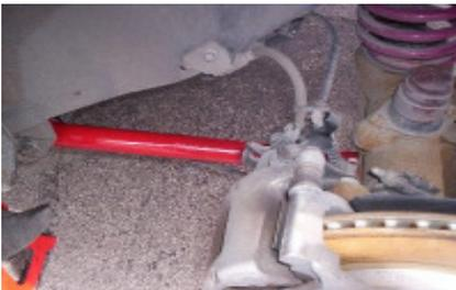
Step 8. Once the bolts are torqued, you can reinstall the hand brake cables. First, insert the cable into the bracket, and slide the retaining clip into position. Then, pull the cable up and through the brake assembly. Position the cable so it properly sits in the brake assembly.
