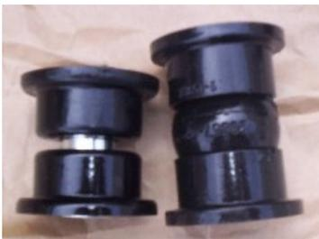
Step 5. Use the supplied grease and generously lubricate the bushings, sleeves, and the inside of the bushing housing on the control arm. Install the bushings into the arm. For the rear bushing, the ball portion goes in the middle, and the outer portions go in next. Then slide the metal sleeve into the hole. For the front, install each side, then the sleeve. The front bushing is not designed with a ball portion, only the outer portions. Correct bushing assembly is shown in the picture below.
