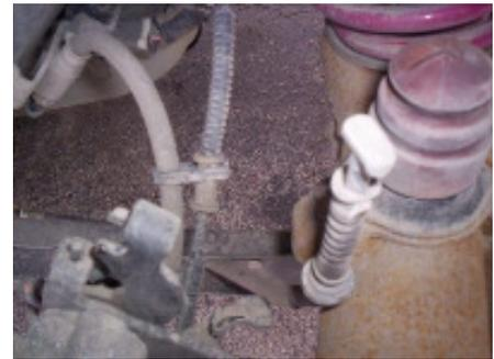
Step 3. Remove the two bolts that attach the lower control arm. One is located at the front of the arm, at the frame rail. The other is located at the rear, on the axle near the shock mount.
