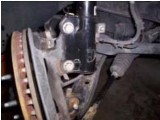
2. Remove the 18mm nut on the strut for the sway bar end link. Remove the end link from the strut by pushing it through the hole. Do Not Use Impact Gun
