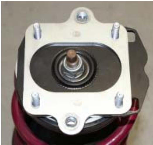
16. We install one 8mm nut onto one of the studs to keep the caster plate in place during shipping. ***Make sure to remove this nut before trying to install the assembly into the car.***
