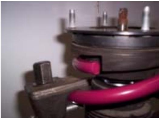
7. Once the spring is compressed, remove the 21mm nut on the top of the strut. You may need to hold the strut shaft with a 10 mm wrench to prevent it from spinning. Once the nut is removed, remove the upper strut mount. We do NOT recommend using impact guns on struts or shocks.
