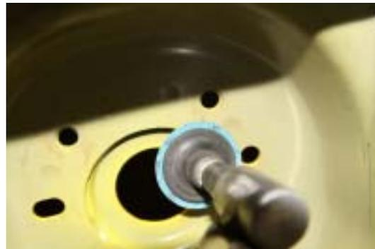
15. The camber plate has an offset bearing design which allows you to install them in a street setting or a race setting. To install in the street setting which will allow you to have more positive camber for lowered cars simply install with the notch toward the inside of the car (engine side) and the race setting you will install the notch toward the fender (outside) of the car.
