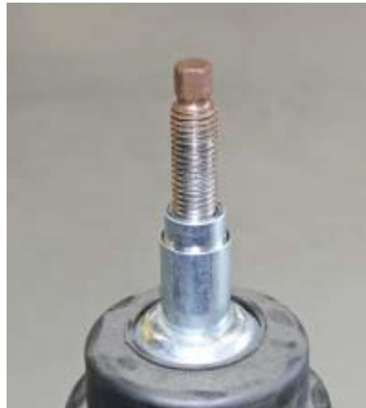
10. Place the camber plate assembly with the spring seat over the strut shaft like shown. Strut not shown for clarity. NOTE: OUR NEW DESIGN DOES NOT HAVE THE SPRING LOCATOR AS THE SPRING IS LOCATED OFF THE STRUT.
