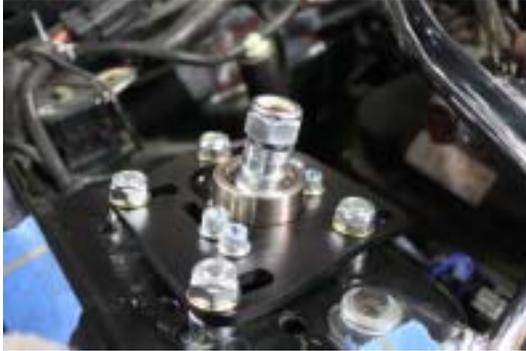
19. The original strut-to-spindle bolts and nuts can now be re-installed and torque to spec. Don't forget to secure the ABS bracket and line, if your Mustang is equipped with ABS.
