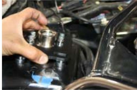
16. Loosely secure the caster/camber plate and bearing cup assembly with the J&M supplied washers and lock nuts. Leave loose to allow for adjustment.
