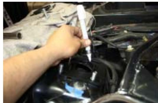
12. J&M supplies various strut spacers of different lengths to accommodate different ride heights. Most lowered Mustangs will require one “tall” strut spacer directly on the strut shaft itself as shown in the picture. The remaining strut spacers will be used at a later point. This combination will maximize suspension travel.
