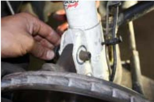
20. At this point, the top strut nut can be tightened to the strut manufacturer's specification (DO NOT USE AN IMPACT GUN.) Go back and double check that all mounting hardware is tight. Double check your preliminary alignment settings.
