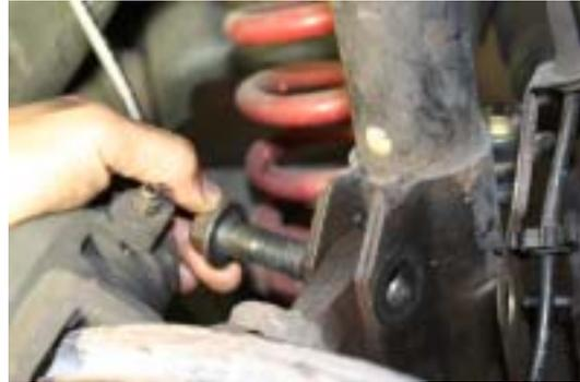
5. Loosen and remove the upper strut mounting nut. Do not use an impact gun. If you are re-using the same struts, you will need to re-use this nut that was just removed. If you are installing new or different front struts, a new nut may be supplied by the strut manufacturer.
