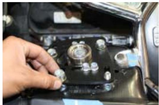
17. Position the caster/camber plate and bearing cup assembly such that the strut will align with the marks you made on the masking tape in step 1. Now all the caster/camber plate and bearing cup assembly bolts can be tightened.
