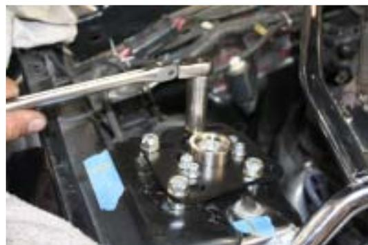
18. The strut can now be installed through the bearing cup in the caster/camber plate assembly. At this point, the remaining strut spacers can be installed on the threaded shaft of the strut. In our case, we used 2 “medium” length strut spacers and 2 “short” spacers per side on the top-side of the strut. Lastly, the top strut nut can be installed. Leave this loose for now.
