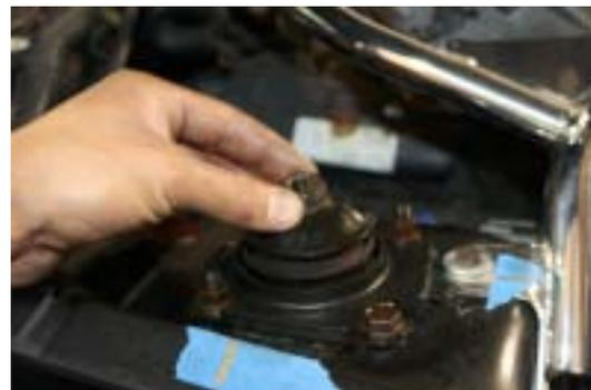
6. With the upper strut mounting nut removed, the stock upper strut mounting components can be removed and discarded as they will not be used.
