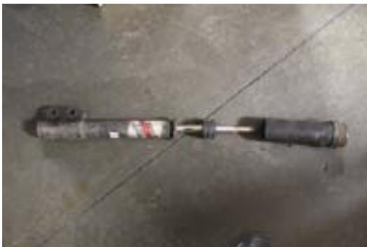
10. On this car, Tokico front struts are being installed in place of the original struts, making it necessary to remove the stock rubber bump-stop from the original strut and transferring it to the Tokico strut. If you are re-using your original struts, retain the bump-stop in its original location. The bump-stop is the only part that gets re-used.
