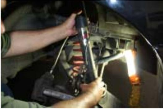
8. The three nuts that secure the top strut plate to the shock tower can now be removed and discarded as they will not be re-used. Often times, the top strut plate is also riveted onto the strut tower. If so, simply drill-out or chisel-off the rivet head to allow complete removal.
